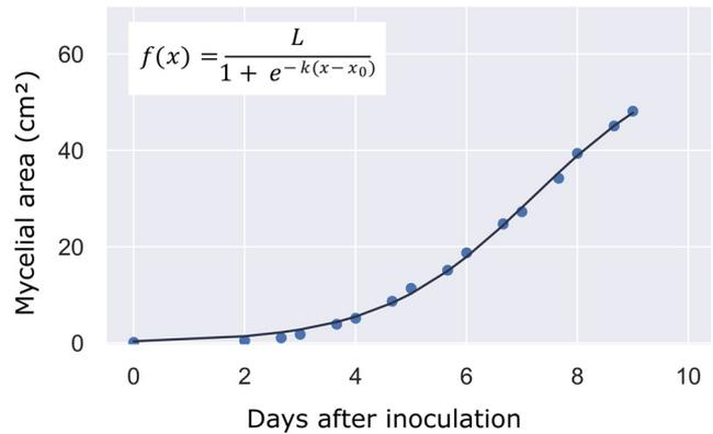
**Figure 1:** Logistic growth curve fitted to mycelial development of *Coniophora puteana* growing on a paste of *Pinus sylvestris* sapwood.  $L$ , the curve's maximum value;  $k$ , the logistic growth rate or steepness of the curve.
