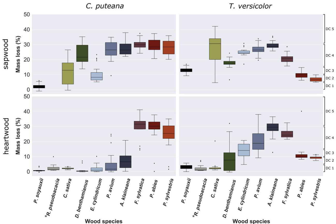
**Figure 4:** Mini-block test: mass loss after 10 weeks of fungal degradation by *Coniophora puteana* and *Trametes versicolor*, growing on sapwood and heartwood mini-blocks of 10 wood species. The axis on the right displays the durability classes as described by CEN/TS 15083-1. *\*Robinia pseudoacacia* was excluded from the sapwood mini-block test due to limited sapwood availability.
